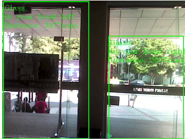
Figure 5. Detection result of a representative scenario. The output information includes object description, location and distance.
