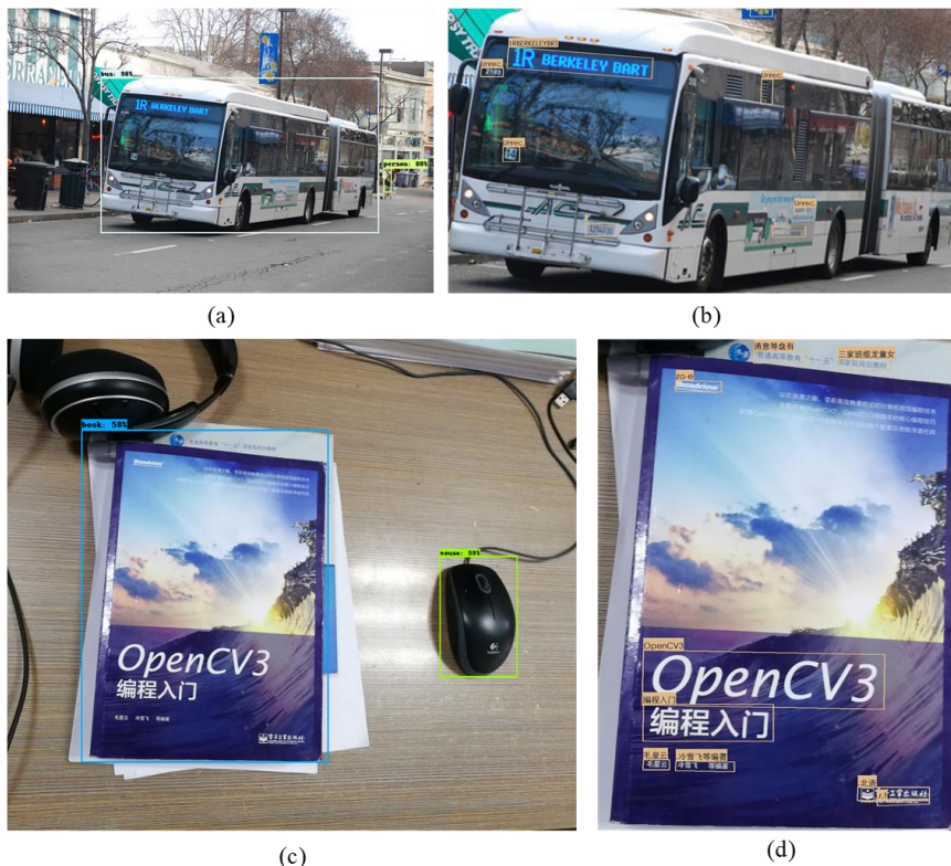
Figure 6. Some examples of the results. A bus and a pedestrian are identified in (a) and text information on the bus is recognized in (b). A book and a mouse are identified in (c) and text information on the bus is recognized in (d). (a) is obtained from COCO2017 datasets. (d) is captured by a mobile phone camera.
