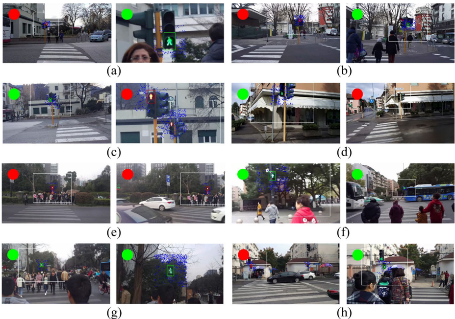
Fig. 11 Some typical PCL detection results of videos in test dataset. a–d represents detection results in video I–IV (Italy dataset). e–h represents detection results in video V–VIII (China dataset). The blue points denote the extracted SURF descriptors
