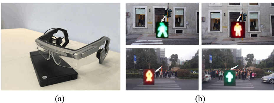
Fig. 1 a Wearable blind navigation system. b Typical pedestrian crossing lights devices in urban areas, and the lamp parts are magnified
