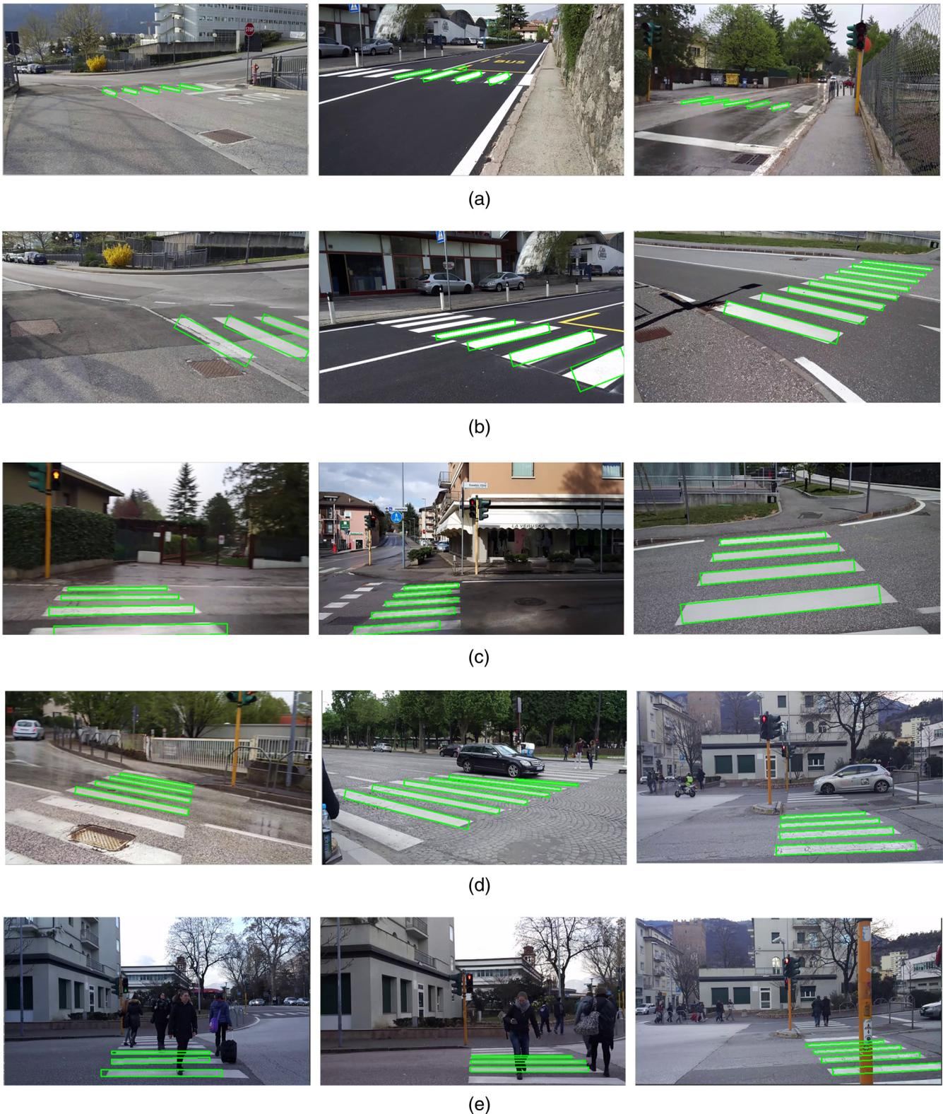
**Fig. 9** Crosswalk detection results using AECA algorithm on testing dataset. The detected stripes of crosswalks are labeled with green borders. (a) The detection results of crosswalks at far distances, (b) the detection results of crosswalks at close distances, (c) the detection results of crosswalks in front of users, (d) the crosswalks detection results in the scenarios of low contrast, and (e) the detection results where crosswalks are partially occluded.
