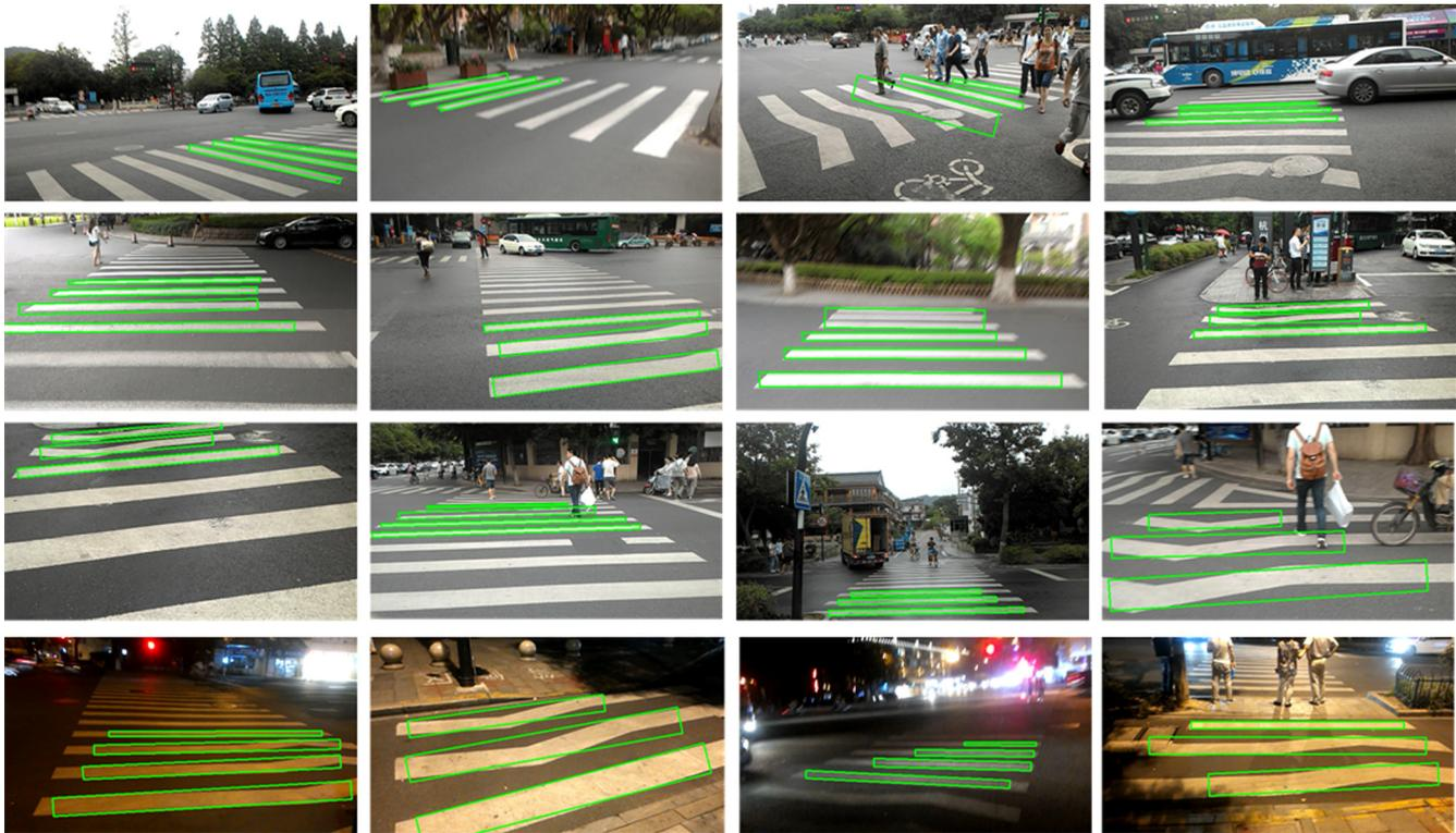
Fig. 13 Crosswalk detection results of field tests.
