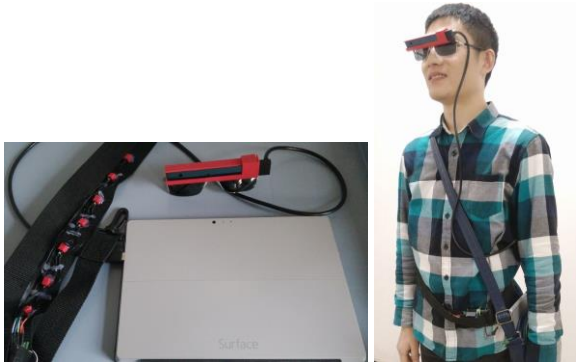
Fig. 12. Experiment device of navigational assistance: the RGB-D sensor, a processor and a vibrating belt.
