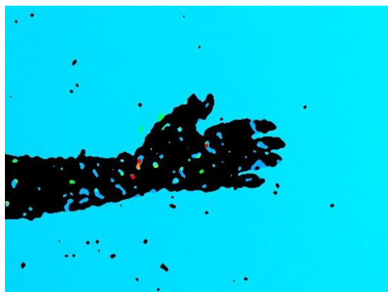
(b) Depth image acquired with Intel RealSense R200. The hand is within minimum range of detection so as to form black holes and mismatching pixels in depth image.
