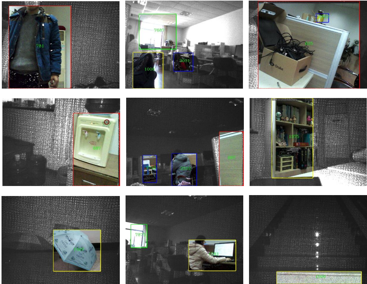
Fig. 11. Obstacle detection from more than minimum range of the sensor: the background is the IR image, and the RGB information of the obstacle is projected using average depth of the object, and the depth in a scale of millimeter is marked in the image. Obstacles of different shapes and locations can be correctly detected.
