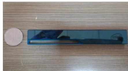
Fig. 1. Intel RealSense R200. The sensor is small and light so it is a good option for navigational assistance from miniaturization perspective.
