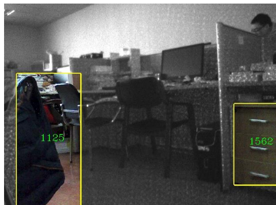
Fig. 7. The obstacle detection with the seeded region growing algorithm. In the IR image, obstacles in the minimum bounding rectangle are replaced with the RGB information, which are projected with average depth. The depth value in a scale of millimeter is marked in the image
