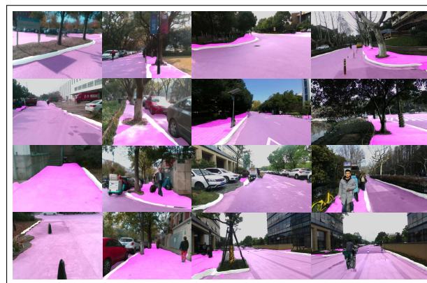
Fig. 9. Diverse qualitative examples of the segmentation of cross-country images (captured in Madrid, Spain and Hangzhou, China) produced by our semantic traversability perception approach with all augmentations. The color masks of road, sidewalks and curbs follow Vistas [7] style.
