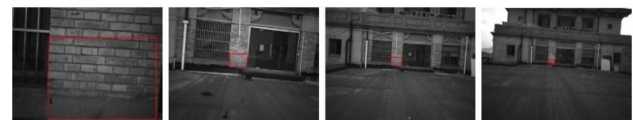
Fig. 14. Four samples of the left images of acquired image pairs. The distances from the wall to the VIAD are 1.066, 6.082, 12.104, and 18.110 m, respectively.
