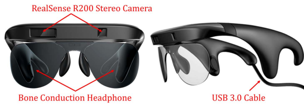
Fig. 8. Intoeer VIAD. Intoeer contains a RealSense R200 stereo camera, a pair of bone conduction headphones, and a USB 3.0 cable, which mainly assists in navigation and obstacle avoidance based on depth maps and images.
