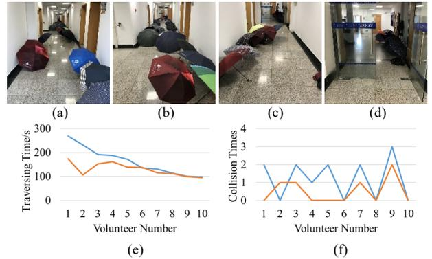
Figure 7. Field test: (a-d) test scenario; (e)(f) experiment data sorted in descending orders of the traversing time while the blue lines are collected with traversability awareness and the orange lines are collected with traversability awareness and low-lying obstacle detection.
