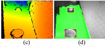
Figure 5. Low-lying obstacle detection and traversable area segmentation: (a)(c) Depth maps in fake color; (b)(d) Low-lying obstacle detection results by producing bounding windows and traversable area segmentation results by producing the green mask to overlay on the IR images.
