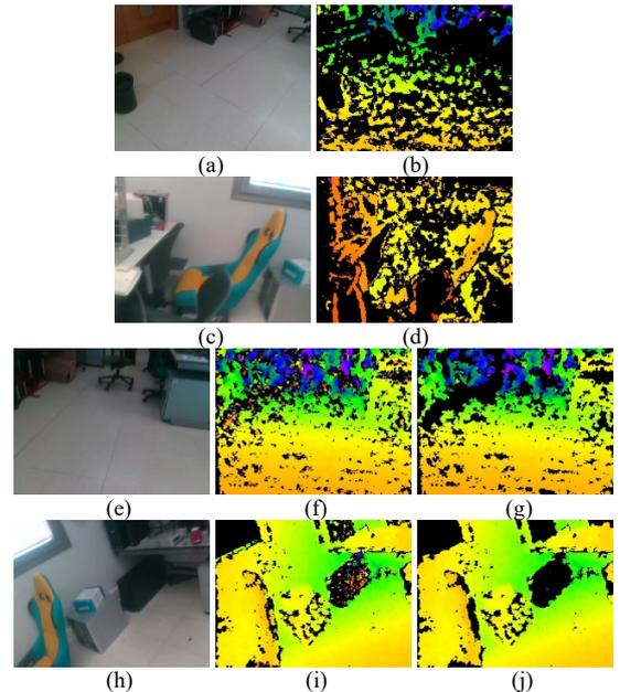
Figure 3. Color images and depth maps from the wearable smart glasses: (a)(c)(e)(h)Color images; (b)(d) Original depth maps; (f)(i) Depth maps with dense preset configuration; (g)(j) Denoised depth maps.
