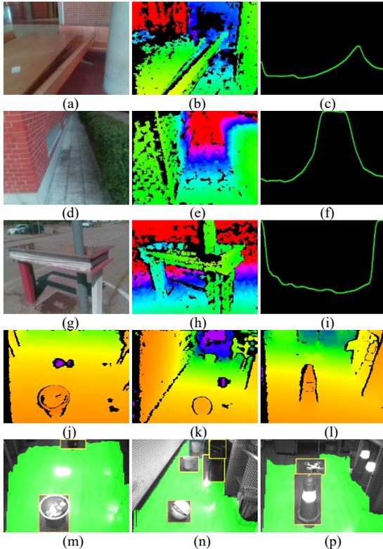
Figure 6. Detection results: (a)(d)(g) Color images of scenarios in both indoor and outdoor environments; (b)(e)(h)(j-l) Depth maps acquired with the smart glasses and the waist-worn pathfinder; (c)(f)(i) Traversable lines; (m-p) Traversable area and low-lying obstacles segmentation results.
