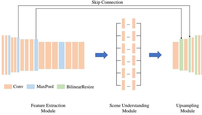
Fig. 2: Overview of the proposed PADENet architecture.
